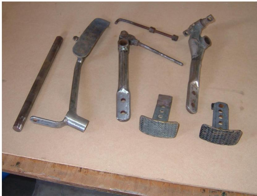
**Components of the pedal system laid out after cleaning and grinding all the non original welds. February 2007. Parts will be carefully stored for nickel plating at a later date. The anti slip mesh welded to the pads can be seen.**
