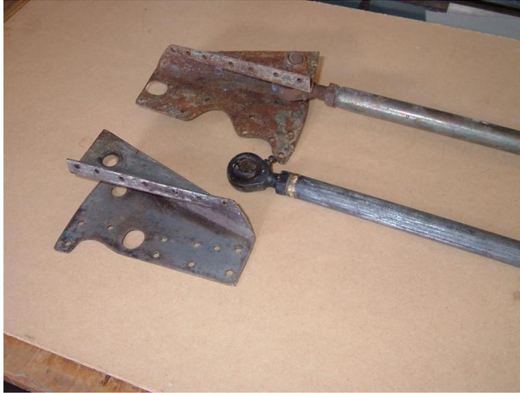
**Radius rod and brackets before and after cleaning and straightening. The spherical joints will all be replaced. Brackets will be painted and later pop riveted to the monocoque and radius rods will be nickel plated. Note that the brackets are opposites and are not exactly the same.**
