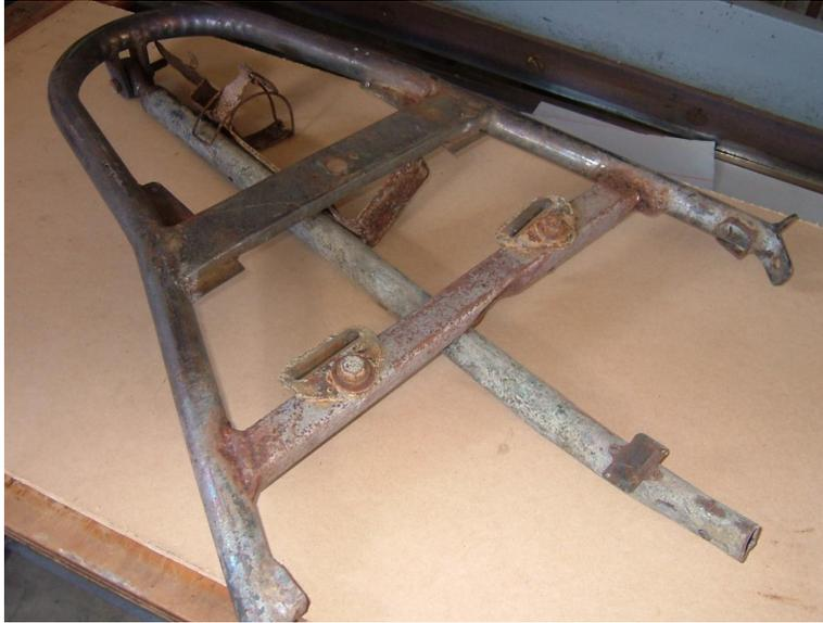
**There's nothing pretty about this. The roll bar has been welded, bent, and neglected. It will be cleaned and prepared but most likely will have to be replaced to meet current safety regulations. There must be a better place for the fire extinguisher bracket.**
