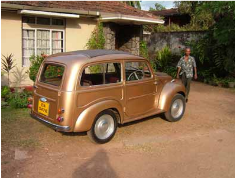
This Fiat Topolino has been in continuous use for over forty years. The 500C Giardiniera model was built from 1949 to 1955. The 569 cc four cylinder engine produced about 17 hp.
