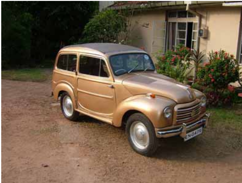
Those wheels are 4.25 x 15 inch, with a 6 ft 8 inch wheelbase. The 500C was the first Fiat to offer heater/demisters.
